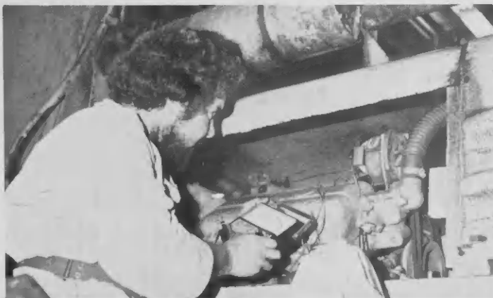
H. Rosel, testing a crane alternator.
